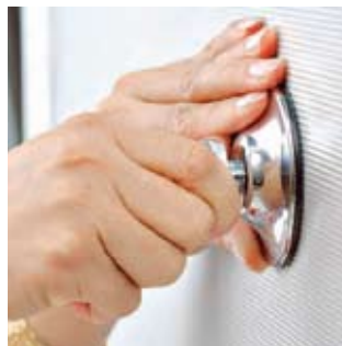
2. Push the suction pad against the surface and tighten the locking bracket
